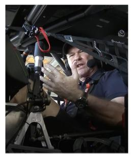
This sequential gear selector, on the left near the drivers fingers, is bolted/screwed to the car floor and appeared to come away fairly easily, at least for a few unlucky drivers.
